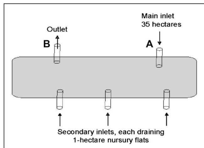
Fig. 2. Schematic diagram of pond at VTS-2, with sampling stations A and B. The pond is 70 m by 12 m × 1 to 2.5 m deep.
